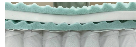
Adhesive (hot melt) method
